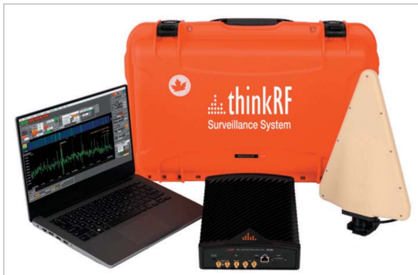
2. The Surveillance System developed by thinkRF includes real-time spectrum analyzers, a laptop, IP networks for multi-sensor deployments, Kestrel's TSCM Professional Software, omnidirectional antennas, and a carrying case for field deployments.
